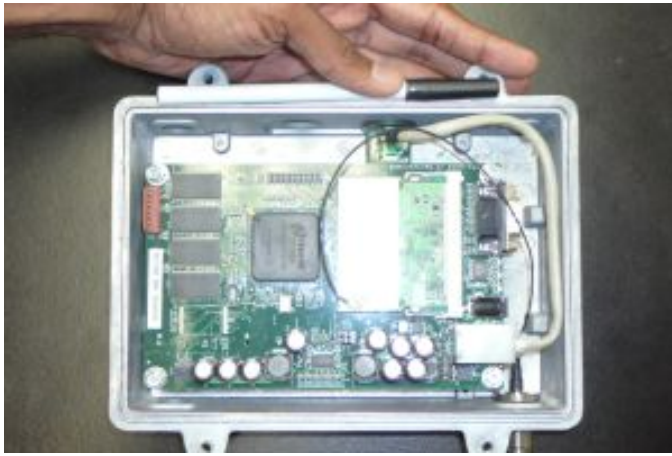
Fig. 4. The inside of the WRAP platform. The hand and the pen in the picture show how small the WRAP board is.
