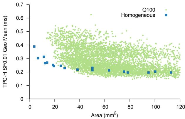
Figure 8: Performance/Area comparison of homogeneous and Q100 implementations
