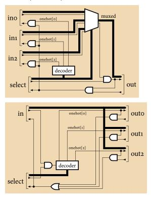
A multiplexer takes a *select* input and uses it to steer the data and *valid* signals from the selected input to the output when *select* is also valid. If the downstream is ready, the token on *select* and the corresponding input is consumed.
