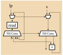
Because information only flows one direction between the loops (i.e., from the lp loop to the s loop), inserting buffers on the channels between decouples the two loops, allowing the lp loop to race ahead and start reading the next list element before the addition operation has been completed. This is exactly pipelining: the next invocation of *sum* starts before the previous one has completed. Townsend [31, §4.5.2] explores how the presence of such non-strict functions improves performance.
