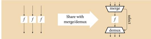
Here, three calls to a function f share a single functional unit for f. A nondeterministic merge node selects and delivers one input to f and also reports which input won each arbitration on a *select* channel. Once f processes the input, a demultiplexer block routes the result back to the appropriate call site based on the *select* token.
