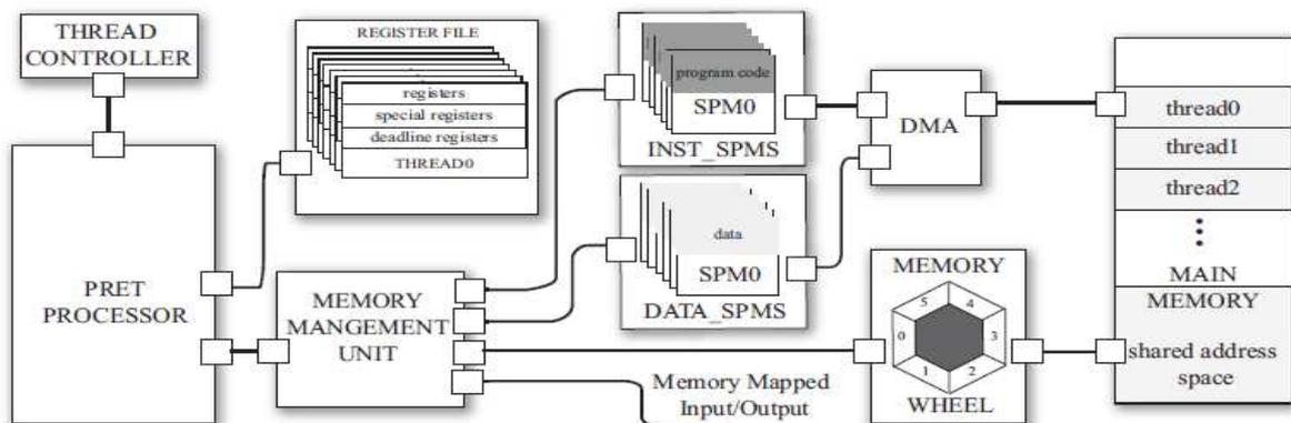
**Figure 2: Block diagram of the PRET Architecture**
