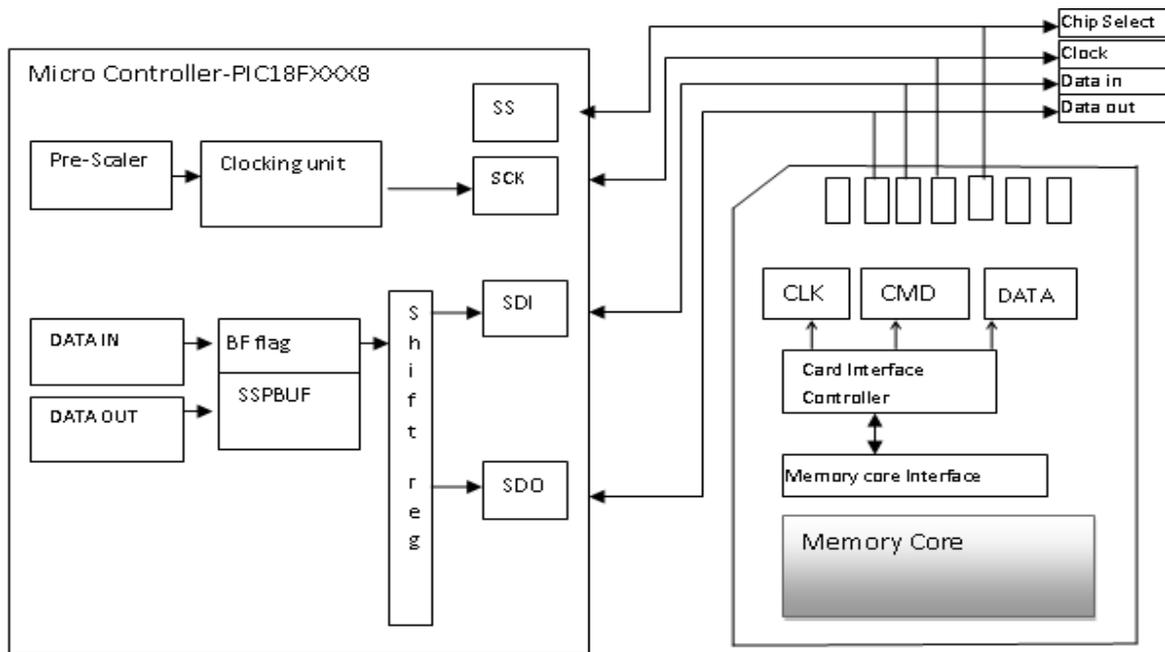
**Figure 1: Block diagram of communication between MMC card and a microcontroller using SPI**
