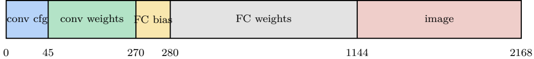
Figure 14: Contiguous 32-bit word layout used by the HPS tools. The figure is drawn for readability; exact word counts are listed in Table 9.
