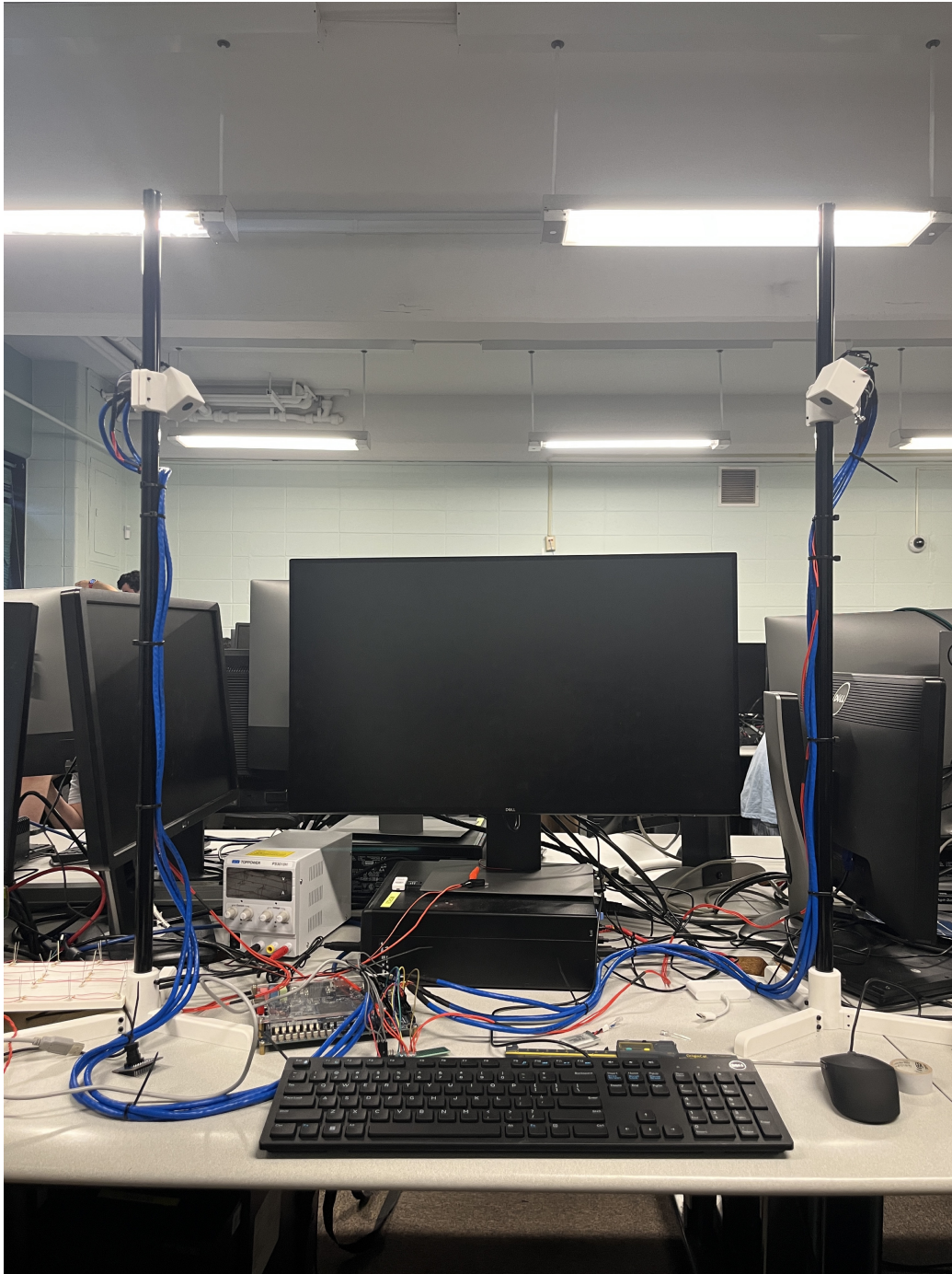
Figure 4: Full setup. Custom camera mounts were designed and printed; Cat 6 cables were spliced and repurposed for fast PCLK-domain signals, with each twisted pair carrying a signal and return ground.
