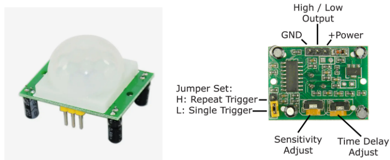
Figure 8. HC-SR501 PIR sensor
