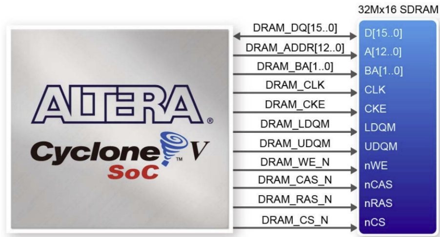
Figure 5. Connections between the SDRAM and the FPGA
