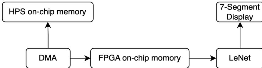
Directory memory access (DMA) is a feature of computer system which allows data to be transferred between device. We use the DMA to transfer data from HPS to FPGA.
