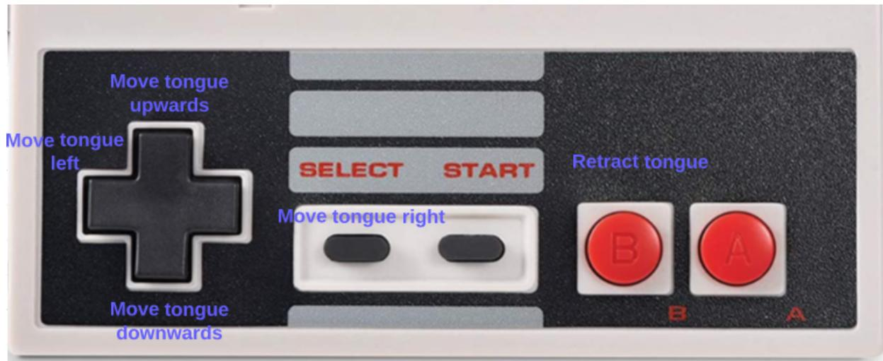
Figure 11: NES USB controller with how they were mapped to be utilized
