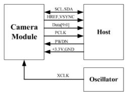
Pinout of Camera Module:
