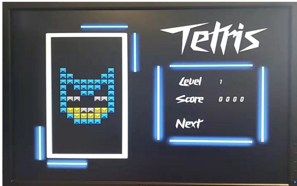
The team made very careful design on the image files since the space of BRAM is very limited. The team used a tile-and-sprite method to do our graphic display. The system has 3 layers in total: background image, blocks and numbers. Background image is still while blocks and numbers will change according to the data stored in registers.
