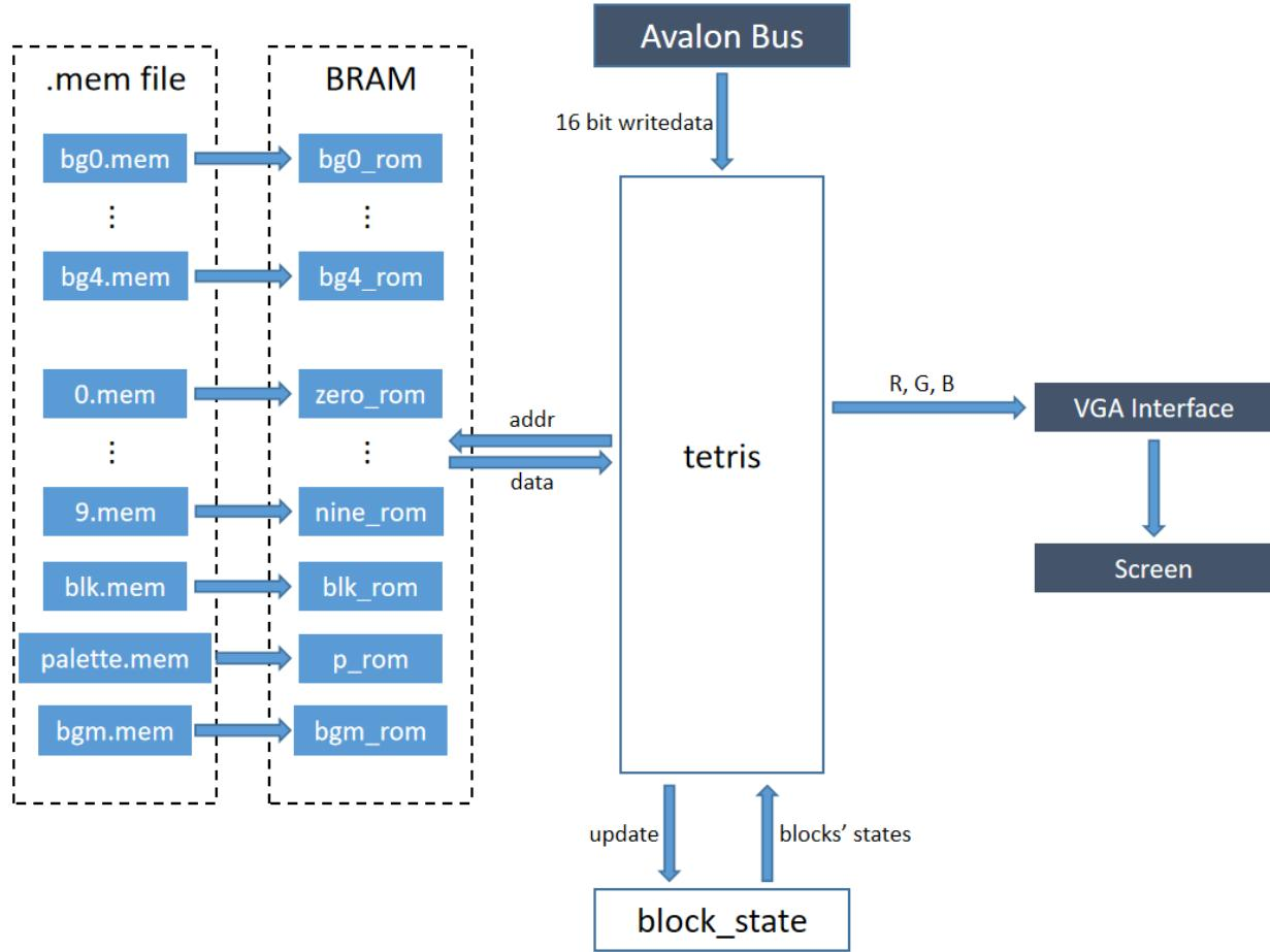
Above is the diagram of our hardware. The team implemented asynchronous ROMs to read the .mem files and store them. Because of different image sizes, the team used addresses of different lengths. Data lines have different lengths as well.
