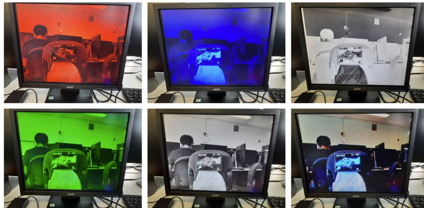
Fig 19. Demo for various Video Processing Modes in following order: Red Filer, Blue Filter, Invert Video, Green Filter, Grayscale Video, Low Brightness.
