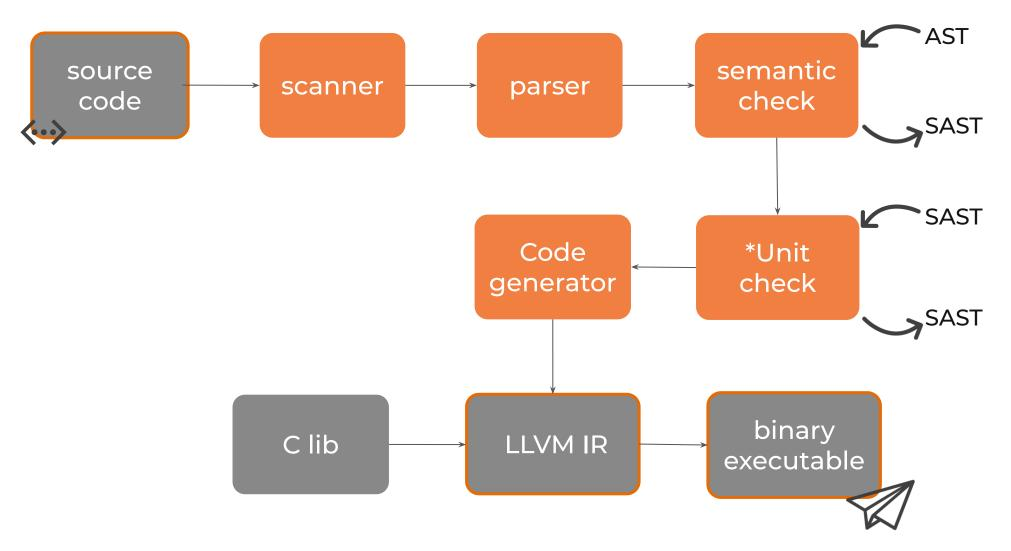
Focus on the normal semantic check like type check and expr validation. Walk over AST and generate SAST.
