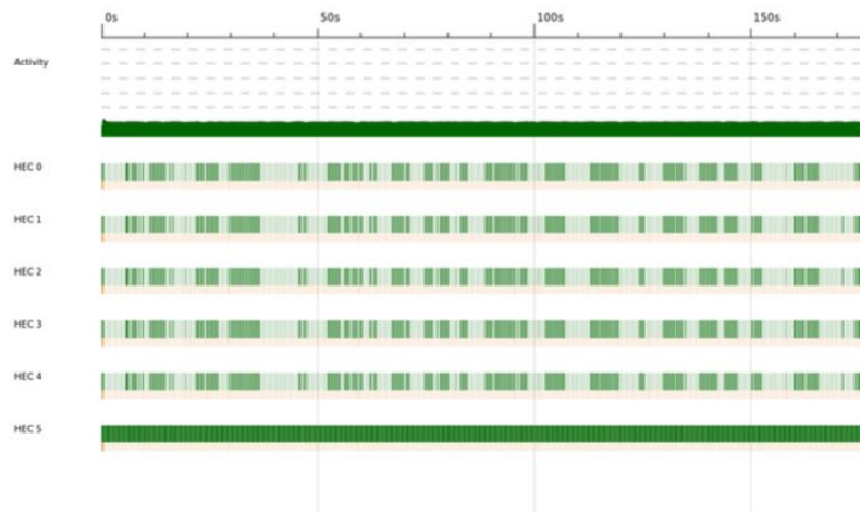
Fig. 4. Threadscope output of parallelized Gradient Descent Algorithm (1,000 iterations) with 6144 chunks on a 2 column by 100,000 row input and 6 cores.
