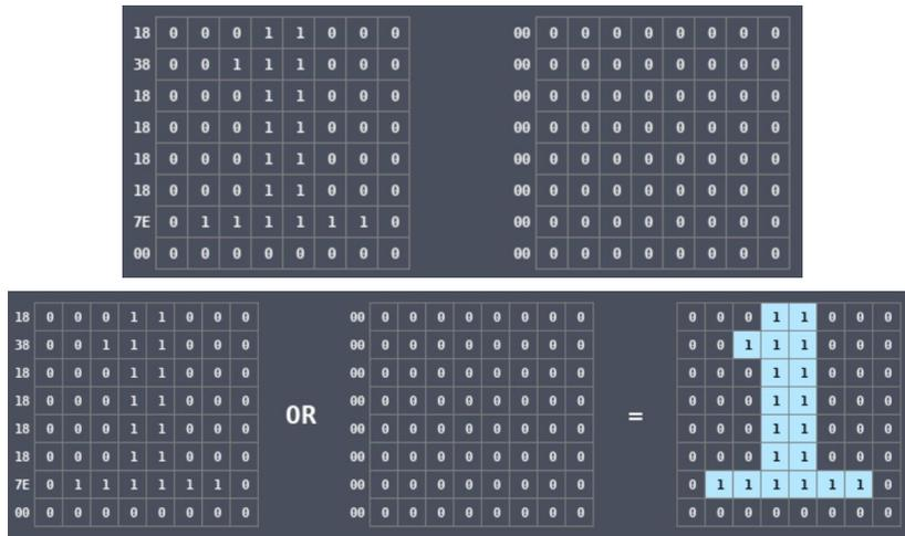
Figure 11. Combining Low and High Bitmap of Pattern Table
