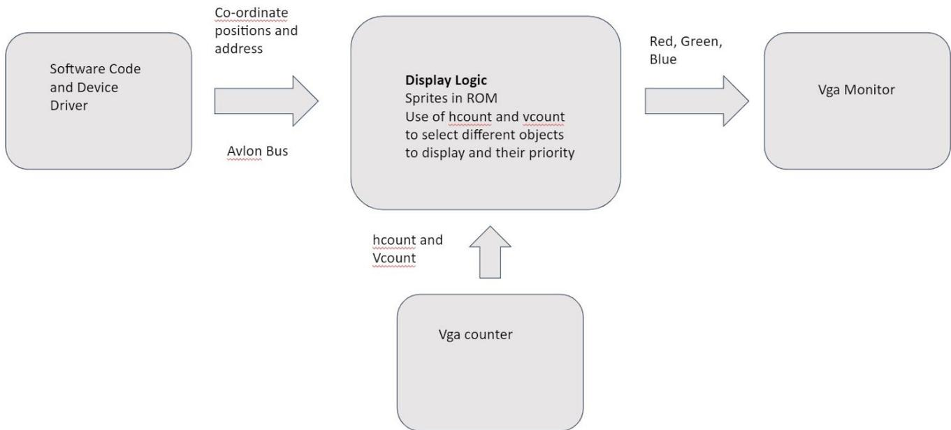
Fig 3. Architecture of SW/HW interface
