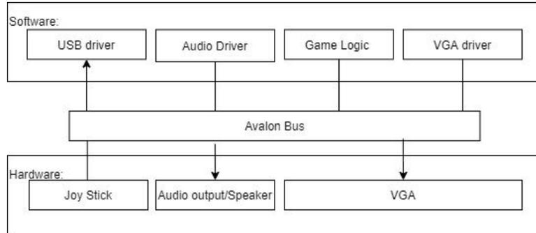
Fig 1. Software & Hardware Interface
