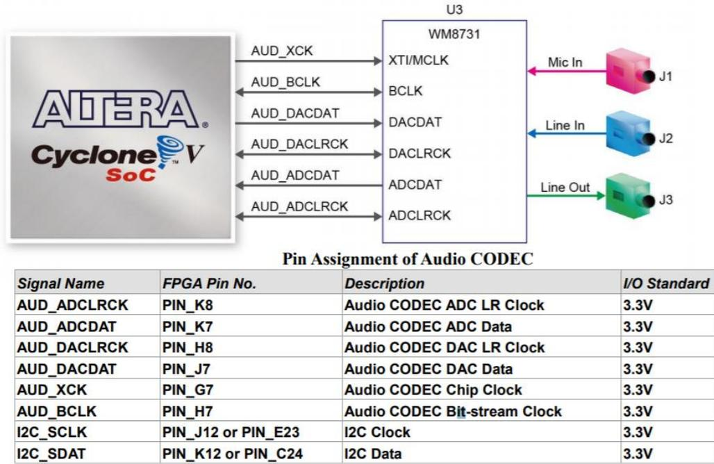
**Fig.7 Block Diagram Connection of circuit**
