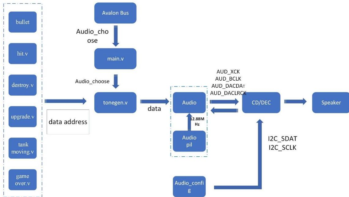
**Fig.8 Audio Module Block Diagram**
