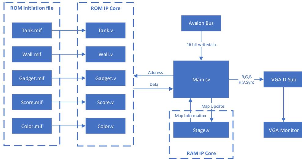
**Fig.6 VGA Module Block Diagram**
