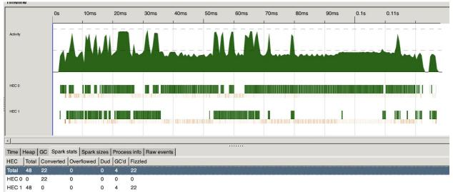
As with the first two tests, there is a small performance speedup from 1 core to 2 cores from 0.166s to 0.137s (17.5% faster). A total of 48 sparks were created in the second core, 22 of which converted in the first core. However, the graph indicates large chunks of time in which the two cores are not being utilized in parallel.
