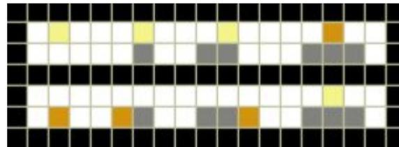
To ensure there was no “columning error”, trapping sand within an 8 pixel wide partition, each tested value was 4 SDRAM words from memory - two from the current row, and 2 beneath it. The second column of chunks becomes the first column of chunks in the next iteration.
