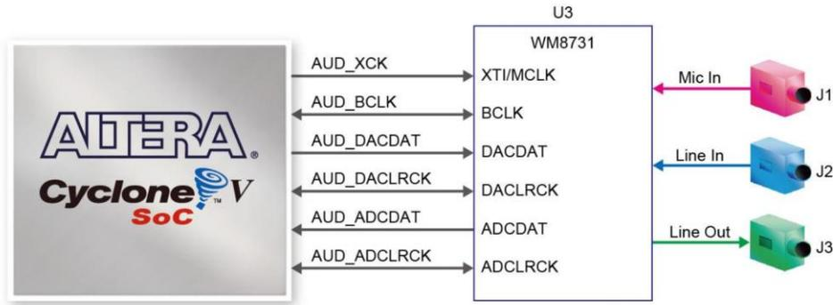
**Fig.5 The connection of the audio circuitry to the FPGA**
