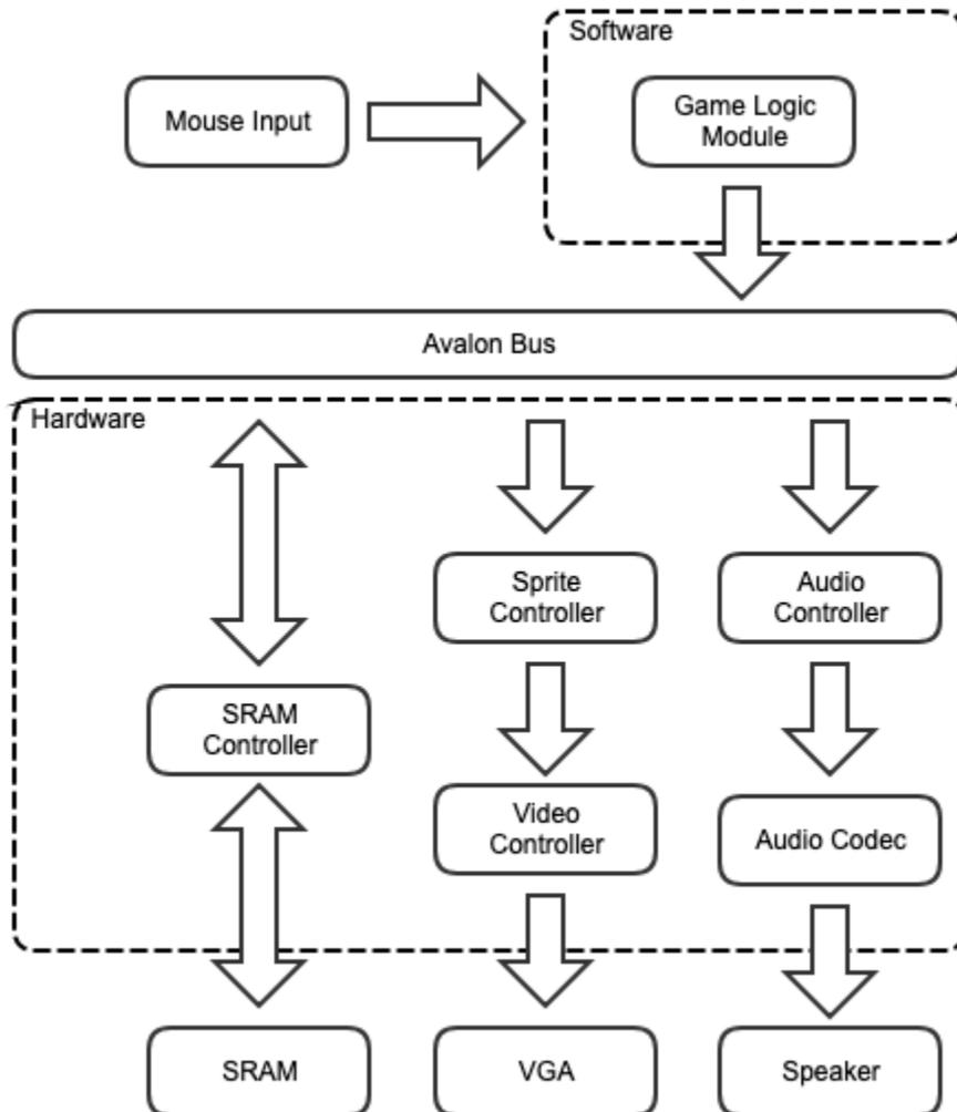
Fig.2 System architecture
