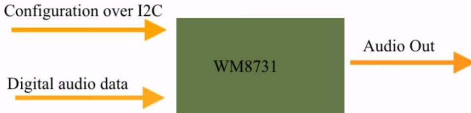
**Fig.7 Block diagram of WM8731 CODEC**
