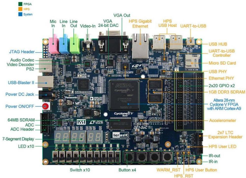
Fig.4 Block diagram of DE1-SoC board
