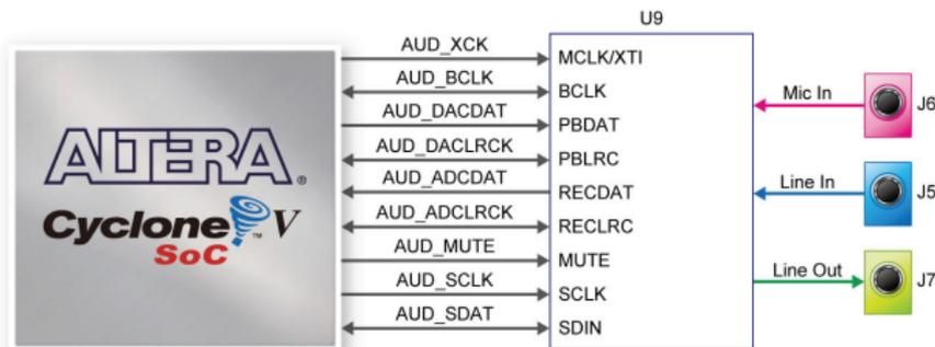
Figure 3-16 Connections between FPGA and Audio CODEC
