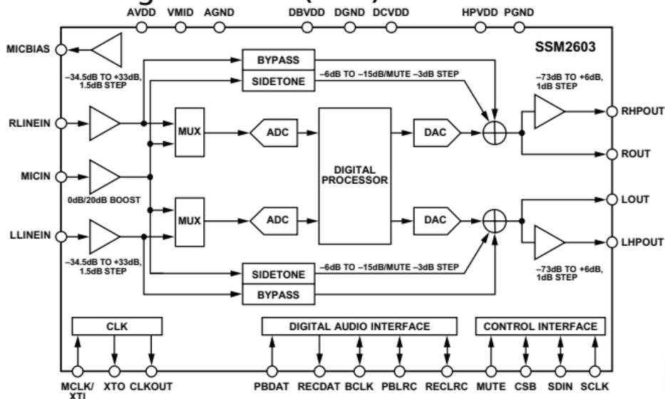
Two 24-bit ADCs; two 24-bit DACs + 7 mW headphone amp
