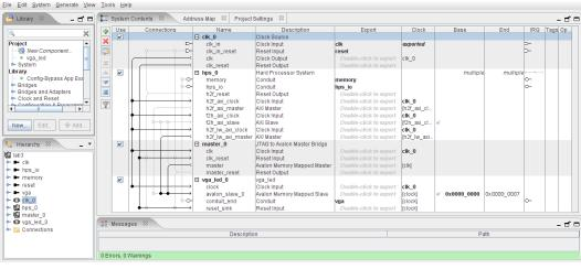
Once you have resolved any errors or warnings, run Generate $\rightarrow$ Generate to have Qsys generate all the files Quartus needs to synthesize to make the design work.
