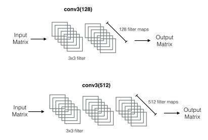
The images go through 5 rounds of convolution. The first round uses 2 sets of 64 filters from the conv3(128) unit. The second set uses the full bank of filters in the conv3(128) unit. The third round uses 3 sets of 256 filters from the conv3(512) unit and the remaining two sets make use of the full bank of the conv3(512) unit.
