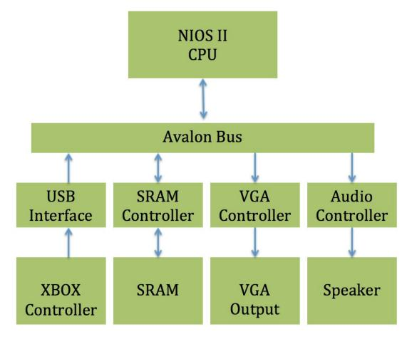
As in the figure, we have a NIOS II CPU and four major peripherals: VGA display, controller, storage part and audio output module. All of above are connected to the Avalon bus so that they could communicate with the NIOS II CPU. For instance, we apply the controller and left click to generate an input signal in the controller and transfer it to the CPU through the bus. The CPU recognizes the input, does the operation and passes the control signal to corresponding peripherals.
