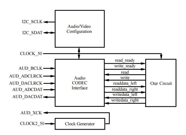
The left-hand side of the above figure shows the inputs and outputs of the system. These I/O ports supply the clock inputs, as well as connect the Audio CODEC and Audio/Video Configuration modules to the corresponding peripheral devices on the board. In the middle of the figure, a set of signals to and from the Audio CODEC Interface module is shown. These signals allow the circuit depicted on the right-hand side to play the background music via speakers.
