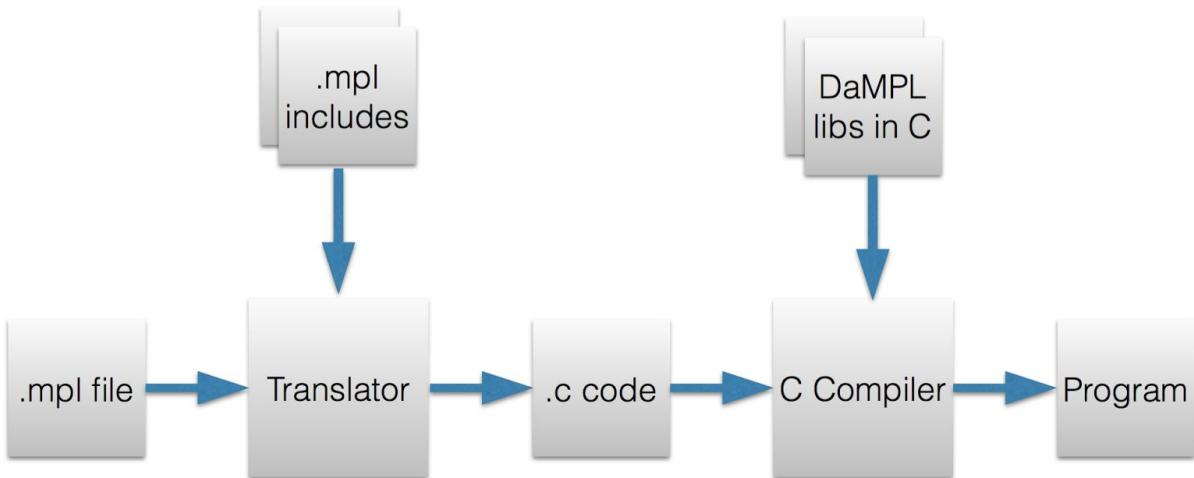
The DaMPL translator takes .mpl files (DaMPL source code) and converts them into a single C code file. Built-in function, as well as array, table and tuple operations are implemented inside the DaMPL libs in C.
