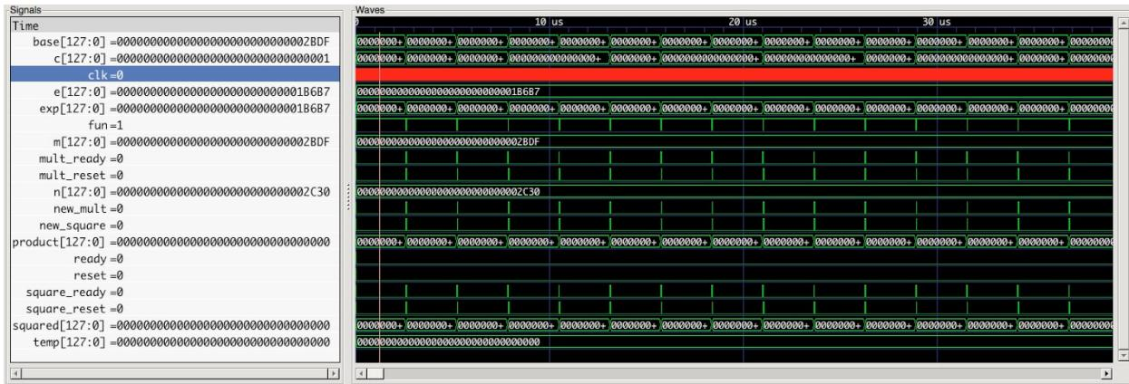
This screenshot from gtkwave demonstrates the timing of the modular exponentiation module. The mult\_ready and square\_ready signals spike each time the multiplication modules finish computing. This then triggers a spike in both the square\_reset and mult\_reset signals, indicating to the multiplication modules that they can safely read the inputs and begin the next iteration.
