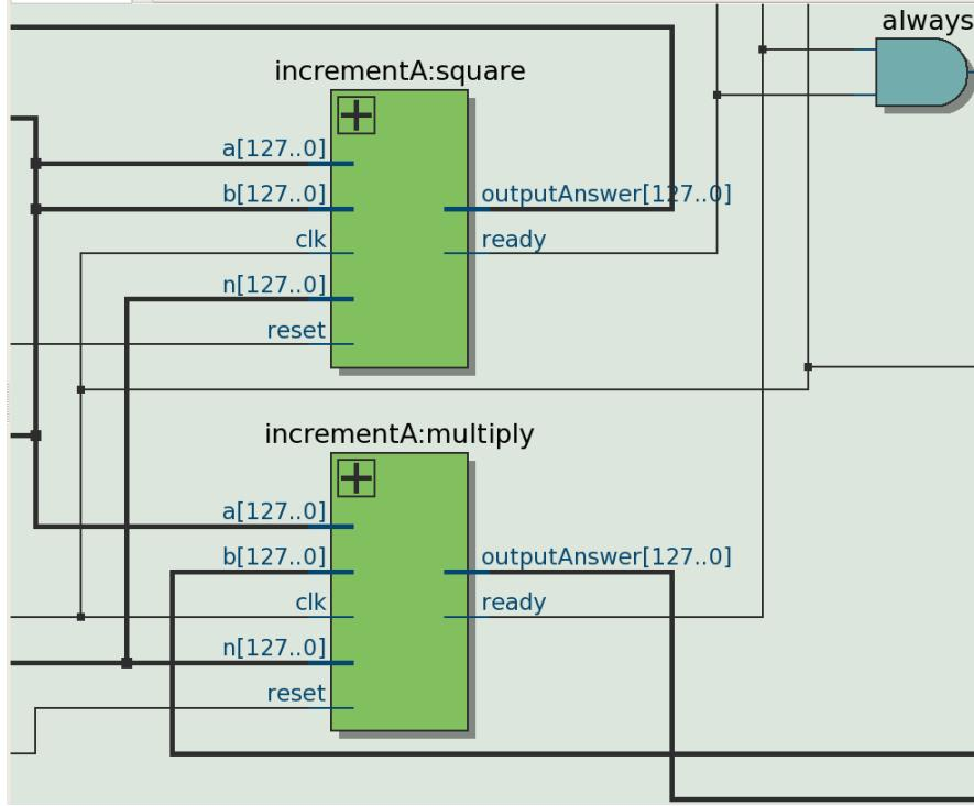
For modulo exponentiation, at each iteration, it checks if the zeroth bit of the exponent is high than the result is set to the result times the base. And if regardless of that result, the base is squared at each iteration with the modulo multiplication. The reduction happens through the modulo multiplication block. Modulo exponentiation is further elaborated in our “Timing Design” section.
