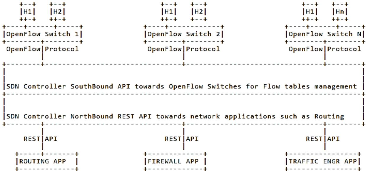
**Figure 1 : OpenFlow architecture is based on so called standard southbound interface between OpenFlow controllers and switches, as well as so called northbound interface between OpenFlow controllers and applications.** Figure 1 the
