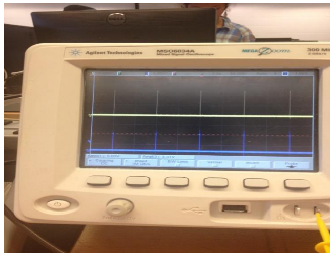
Figure2- Echo and Trigger Waveforms (yellow->Echo Blue->Trigger)
