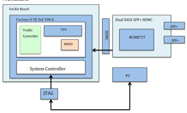
The flow chart is shown as above. The main work will be modify/generate "10GbE MAC and XAUI PHY" part which is marked as "???" and successfully make the SoCKit support XAUI communication.
