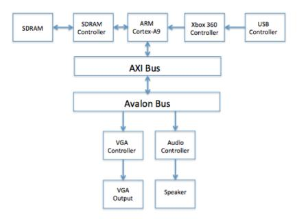
The Avalon Bus communicates between the ARM processor and different peripherals. The Xbox 360 Controller will be connected to the ARM processor through HPS. We will be using the SDRAM on the HPS for memory to store sprite figures and the sound waveforms. VGA and audio output are connected to the FPGA portion of the board through the Avalon bus. The HPS could talk to FPGA through an AXI bus.
