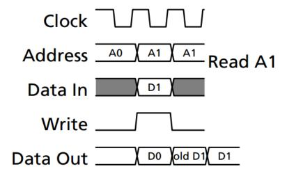
Address is a 16 bit signal that informs the memory which address to access. Data In and Data Out are 32 bits wide, and transfer data between the devices. When write is 1, the memory reads data from Data In into the specified address. When write is 0, the memory writes data from the specified address onto Data Out.
