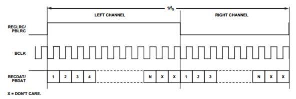
PBLRC is the digital audio frame clock which is used to determine whether the audio data stream is left channel data or right channel data. BCLK is the digital audio bit clock, which informs the device when a new bit is on the data stream. PBDAT contains the time domain multiplexed left and right channel audio stream data.
