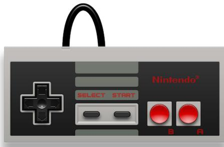
For gameplay, players will utilize all available buttons on the controller. The “up,” “down,” “left,” and “right” buttons on the controller’s d-pad control the direction of the snake. The “select” button can be used to pause the game, the “start” button can be used to pause the game, the “A” button can be used to utilize the “freeze” power-up once it’s attained, and the “B” button can be used to utilize the “edwards” power-up once it is attained.
