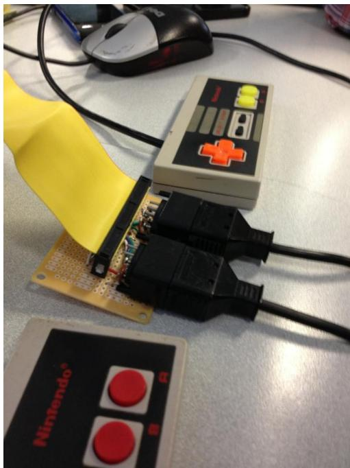
Once the NES controllers were adapted, we constructed an FSM in hardware to interpret the protocol. The NES protocol is slightly unconventional: the state of each button is sent as part of a serial byte. Our FSM is able to determine which button(s) the user pressed, and communicate that to the software. A picture of the protocol is below.
