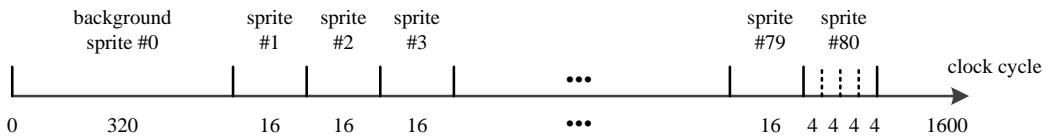
As the figure shows, at the first 320 clock cycles of 1600 cycles, the sprite controller computes the first row of background. And every 16 cycles after the first 320 cycles, the sprite controller computes the first row of corresponding sprites and if it should be shown, overwrites the previous sprites.
