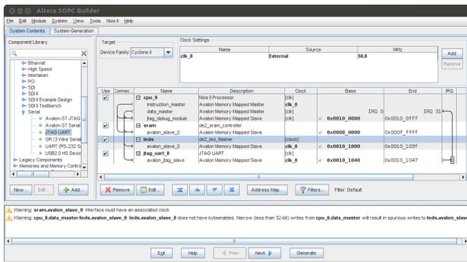
Figure 12: The final configuration of the LED flasher system
