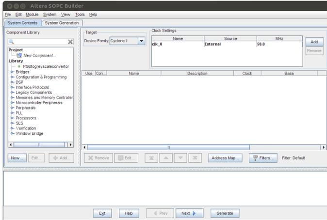
Figure 4: The SOPC Builder main window. Available components are listed on the left.
