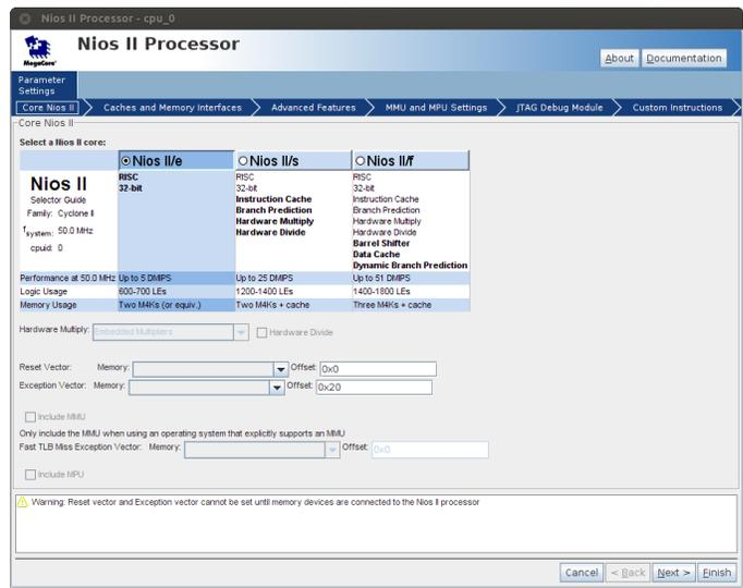
Figure 5: Adding an Nios II processor in SOPC Builder
