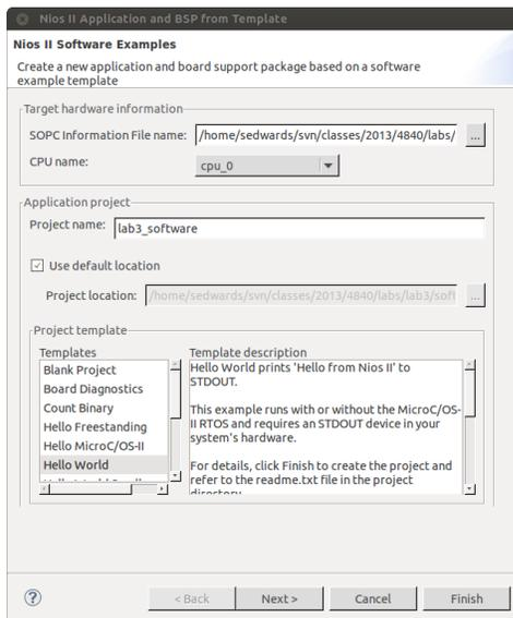
Figure 15: Creating a new application and BSP from a template
