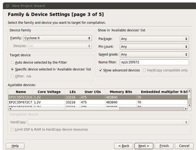
Figure 2: Selecting the device in Quartus
