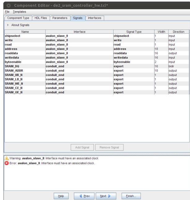
Figure 8: Associating the signals with interfaces
