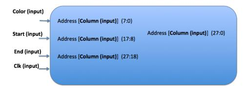
The column generator translates the start position and end position of the wall to be rastered and populates the framebuffer column by column. By using this component we are able to minimize the number of writes that nios processor makes to the framebuffer.
