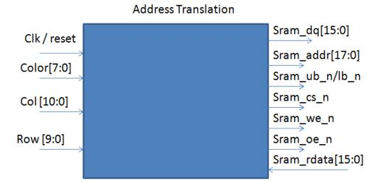
The address translation transmit position information and color information to SRAM buffer. The VGA raster would read data from the SRAM and recalculate it with LUT and generate 10 bit RGB data for VGA. This would allow for storage saving in SRAM, while being compatible with the RGB data for the VGA.
