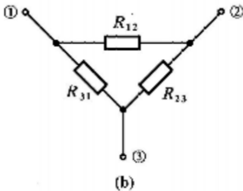
*y configuration(left) and delta configuration(right)*
