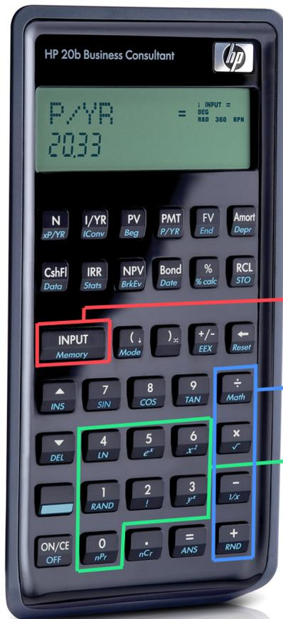
To carry out a simple operation, begin by typing your first operand into the keyboard. Then, press INPUT. The number you entered will appear on the LCD. Next, type out the second operand, and again press INPUT. Finally, press the operator you would like to use. The answer will then appear on the LCD.
