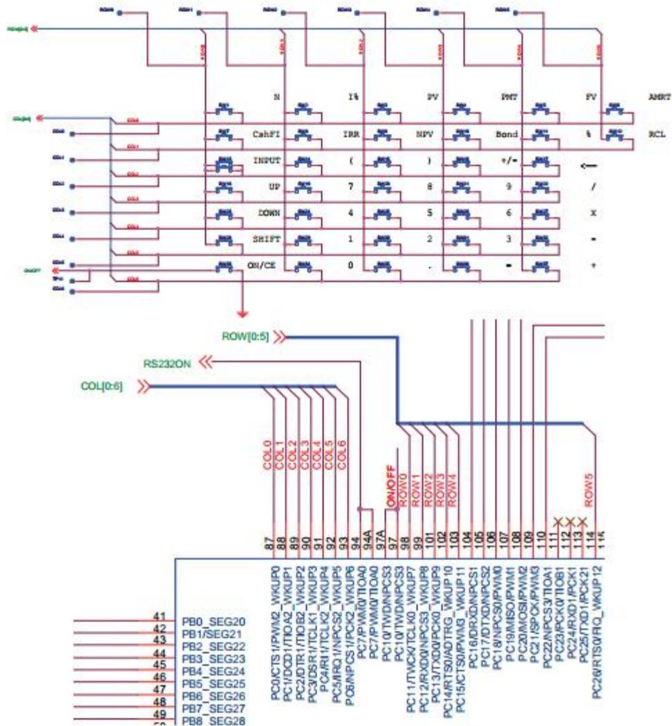
Figure 3: Schematics for the HP 20b keyboard. The top is the keyboard matrix itself; the bottom shows how the matrix is connected to the 8AM71 chip. Note that the ON/CE key is separate (not part of the matrix) and that "columns" of keys are actually horizontal.
