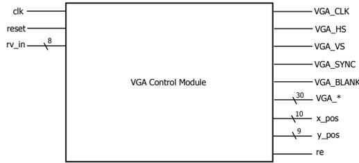
Figure 18: Block diagram of the VGA module
