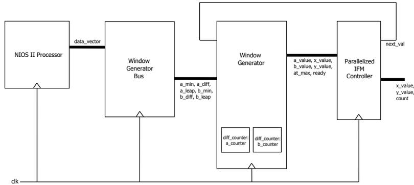
Figure 7: Block diagram illustrating  $(x, y, a, b)$  tuple dataflow.
