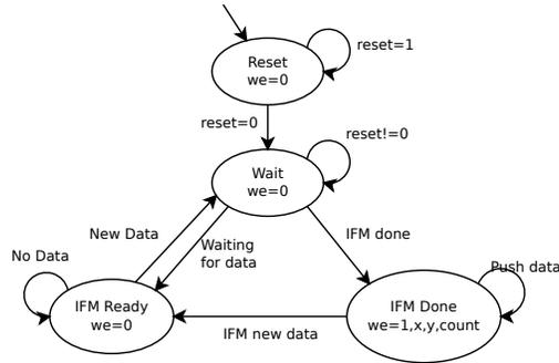
Figure 13: State diagram for a single IFM unit (IFM handler/wrapper), Moore machine: using abstract transition descriptions.
