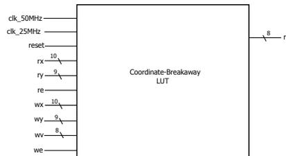
Figure 14: Block Diagram of the Coordinate-Breakaway LUT: signals on the right side are inputs, signals on the left are outputs.
