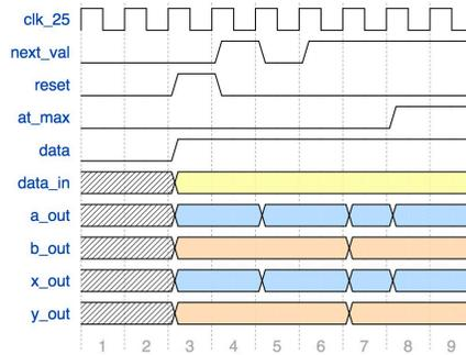
Figure 9: Timing diagram of interface between the window generator and the IFMs.
