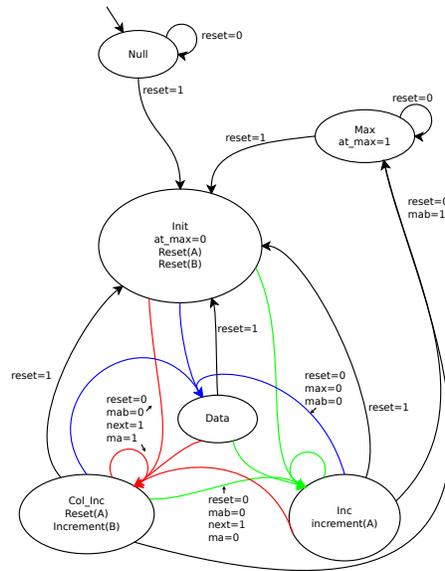
Figure 8: State Diagram for the window generator code, Moore machine: signals  $\text{max}=\text{c\_cuis}=\text{max\_itr}$ ,  $\text{leap}=\text{iter\_count}=\text{v\_leap}$ . Omit unused signals (X) for compactness.
