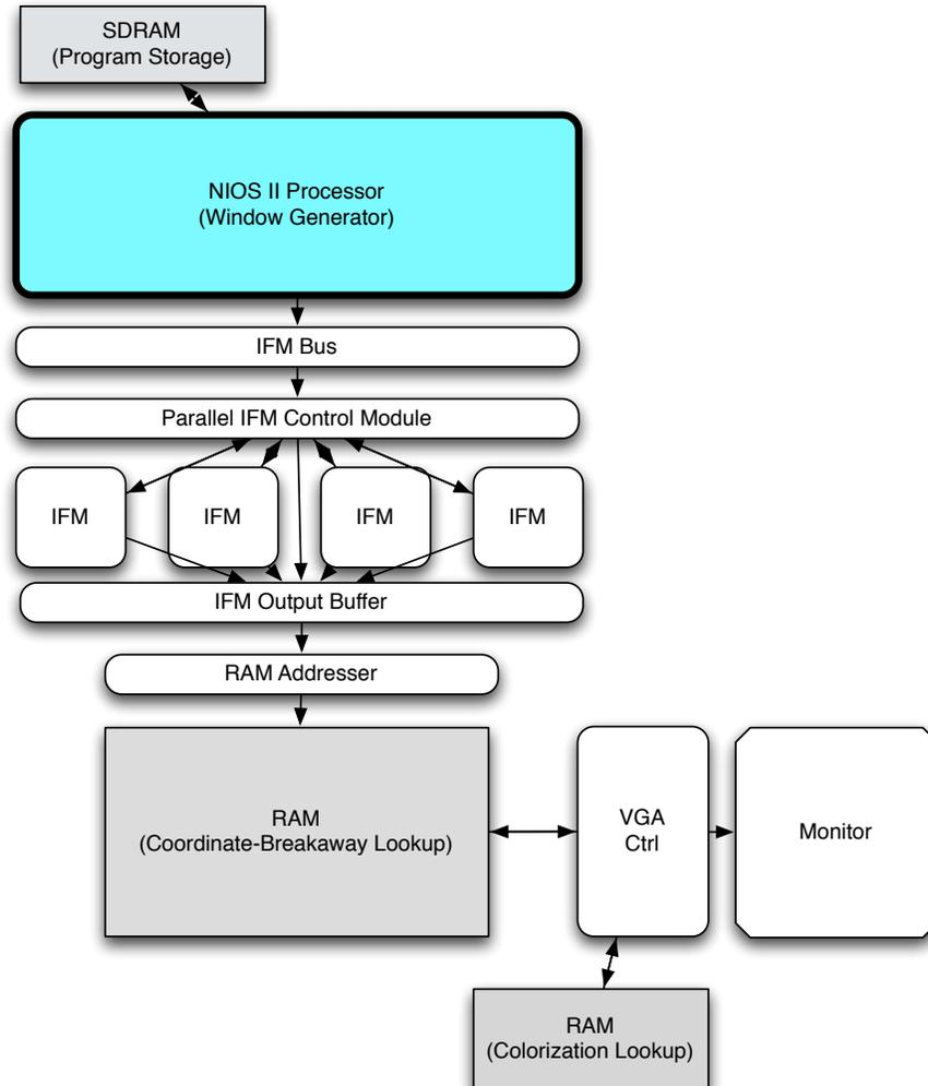
Figure 1: High-level Block Diagram
