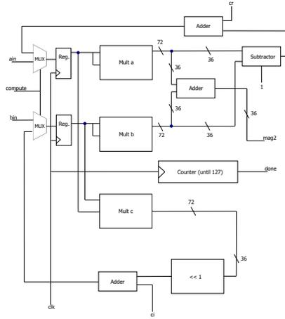
Figure 11: Arithmetic Logic Circuit within each IFM
