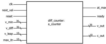
Figure 4: Block diagram of a differential counter used in window generation
