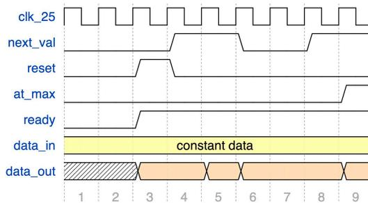
Figure 6: Timing diagram of the differential counter
