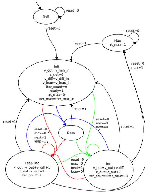
Figure 5: State Diagram for the diff counter, Moore machine: signals  $max=c_{cuis}=max_{itr}$ ,  $leap=iter\_count=v\_leap$ . Omit unused signals (X) for compactness. Colorcoded signal bundles.
