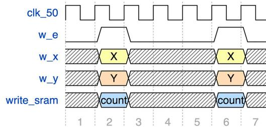
Figure 17: Timing diagram of the interface between the IFMs and the Coordinate-Breakaway LUT.
