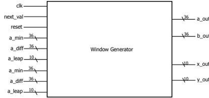
Figure 3: High-level Block Diagram of the Window Generator
