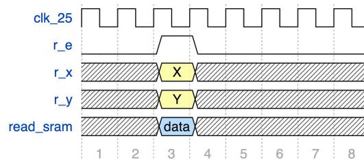
Figure 15: Timing diagram of the interface between the Coordinate-Breakaway LUT and VGA module
