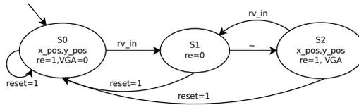
Figure 19: State diagram for the VGA module, Mealy machine:  $\sim$  stands in for no input/output, and VGA stands in for all the VGA\_ signals (VGA\_CLK, VGA\_HS, VGA\_VS, VGA\_BLANK, VGA\_SYNC, VGA\_R, VGA\_G, VGA\_B). Omits unused signals for compactness.
