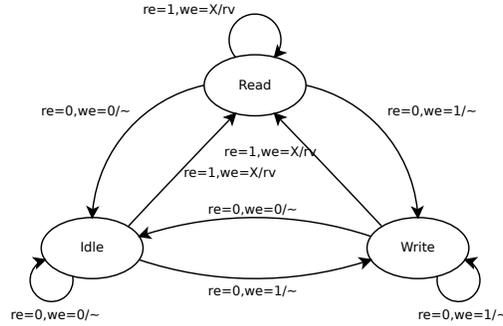
Figure 16: Simplified State Diagram of the Coordinate-Breakaway LUT: Mealy machine, only includes re and we as inputs and rv as an output, with  $\sim$  denoting a lack of outputs
