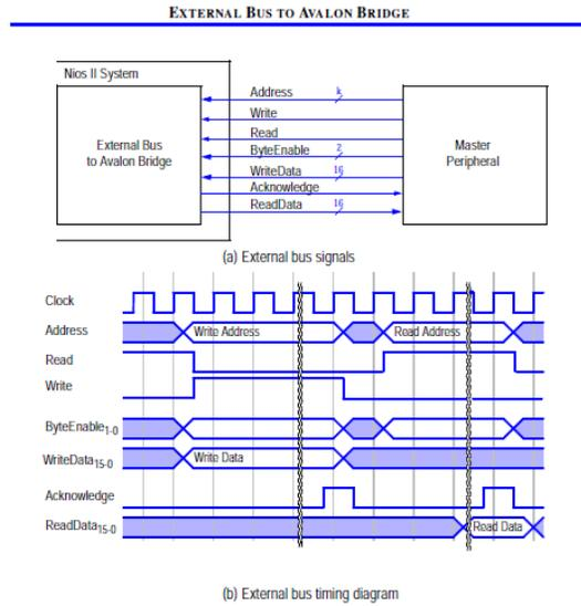
Figure 2: Block and Timing Diagram of the Avalon interconnect fabric. Provided by Altera Corporation.
