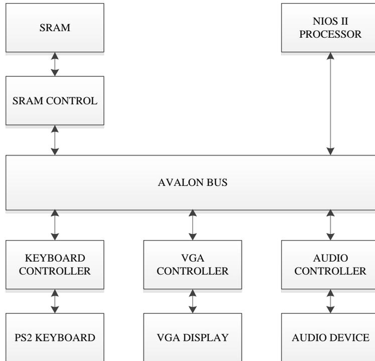
The hardware structure is shown above. As can be seen, we need to build SRAM, NIOS processor, VGA controller, audio controller and keyboard module all connected to the Avalon bus, which makes the communication between CPU, peripheral devices, such as keyboard and LCD display, and Avalon bus come true. This structure is similar to what we have done in lab2 and lab3.
