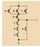
(b) Draw the schematic for a static CMOS gate that implements  $Y = \overline{(A+B)C+D}$
