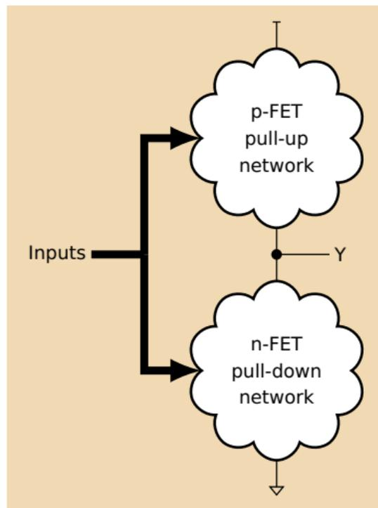
Pull-up and Pull-down networks must be complementary; exactly one should be connected for each input combination.
