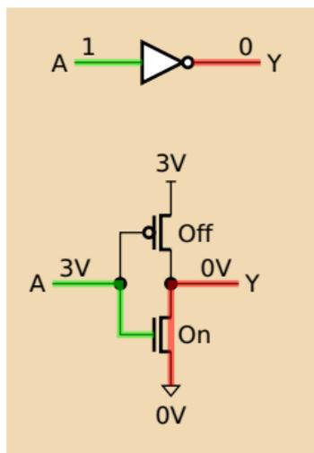
When the input is near the power supply voltage ("1"),
