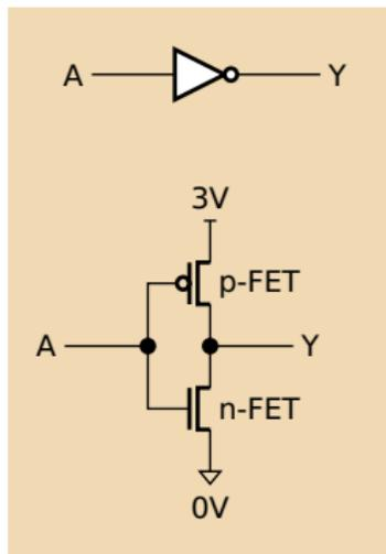
An inverter is built from two MOSFETs:
