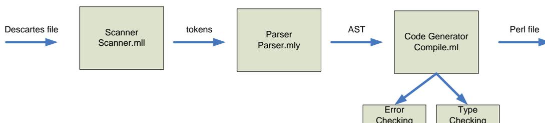
Figure 5.1: block diagram of Descartes compiler
