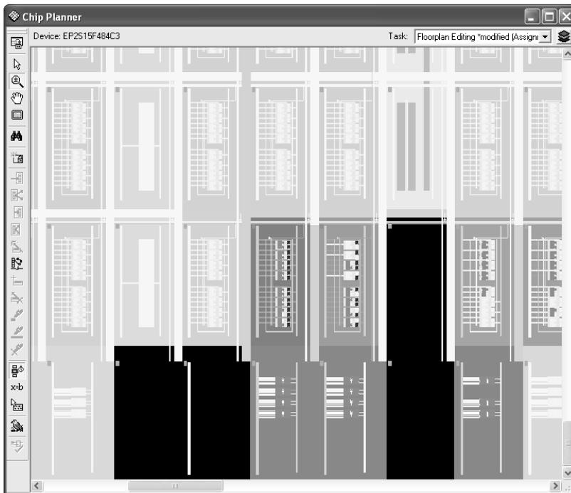
Resource usage in the Chip Planner is color coded. Different colors represent different resources, such as unassigned and assigned pins and logic cells, unrouted items, MegaLAB™ structures, columns, and row FastTrack® fan-outs. The Chip Planner also allows you to customize the floorplan view using filters to show pins and the interior structure of the device.
