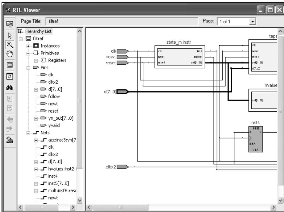
The RTL Viewer displays the Analysis & Elaboration results for Verilog HDL or VHDL designs, and AHDL Text Design Files (.tdf), Block Design Files (.bdf), and Graphic Design Files (.gdf). For Verilog Quartus Mapping Files or EDIF netlist files that were generated from other EDA synthesis tools, the RTL Viewer displays the hierarchy for the atom representations of WYSIWYG primitives.
