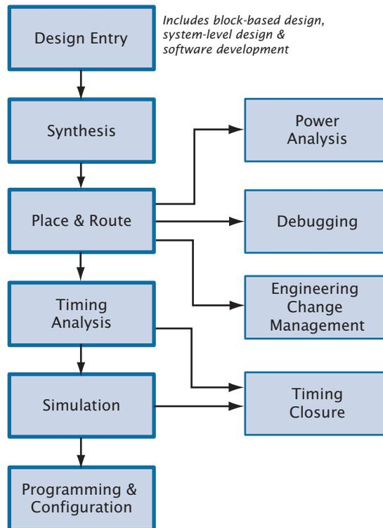
In addition, the Quartus II software allows you to use the Quartus II graphical user interface and command-line interface for each phase of the design flow. You can use one of these interfaces for the entire flow, or you can use different options at different phases.
