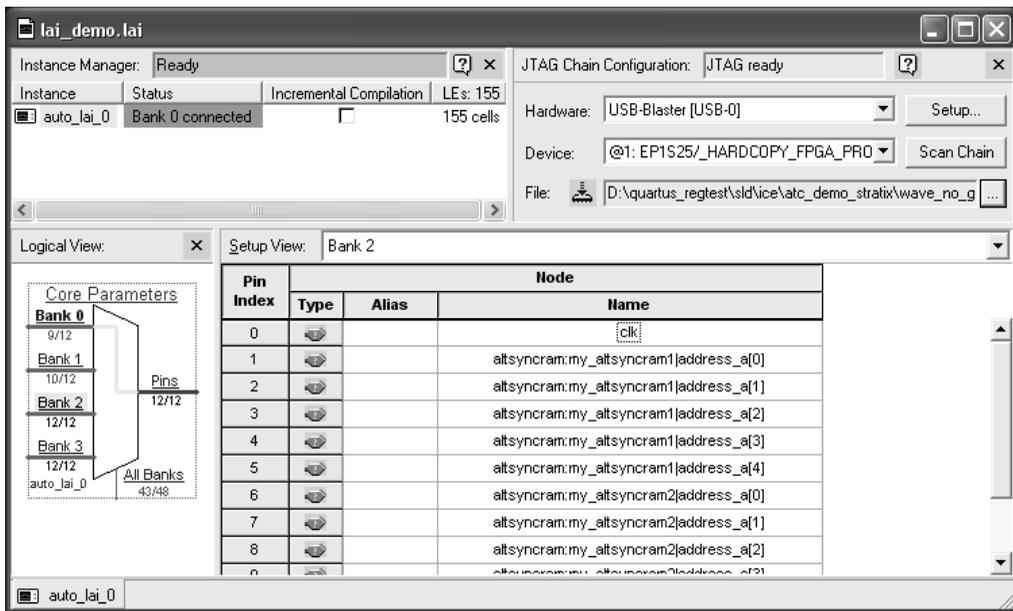
Edit the Logic Analyzer Interface File to specify the number of pins to use, the number of banks to use, and the capture mode. In the **Output/Capture mode** list, specify **Combinational/Timing** or **Registered State**. In the **Clock** box, specify the clock signal associated with the design. In the **Power-up state** list, select **Bank 0** or **Tri-stated**.
