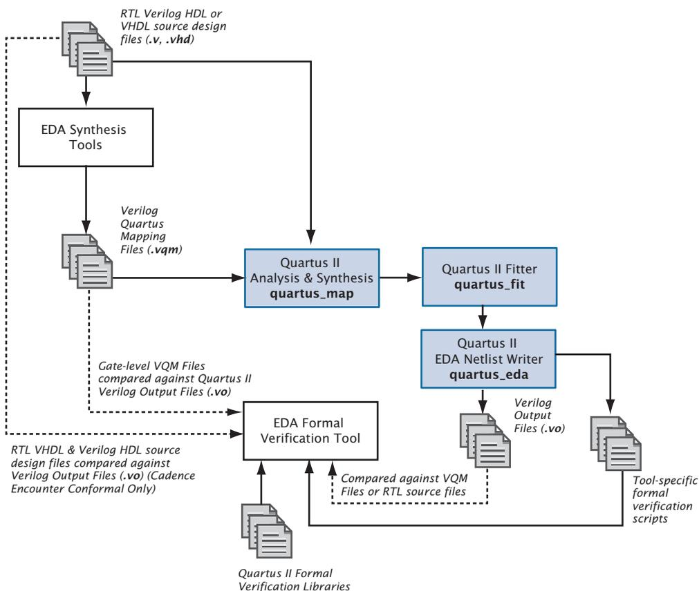
The type of formal verification supported by the Quartus II software is equivalence checking, which compares the functional equivalence of the source design with the revised design by using mathematical techniques rather than by performing simulation using test vectors. Equivalence checking greatly decreases the time to verify the design. The Quartus II software allows you to verify the logical equivalence between the synthesized gate-level Verilog Quartus Mapping Files (**.vqm**) generated by
