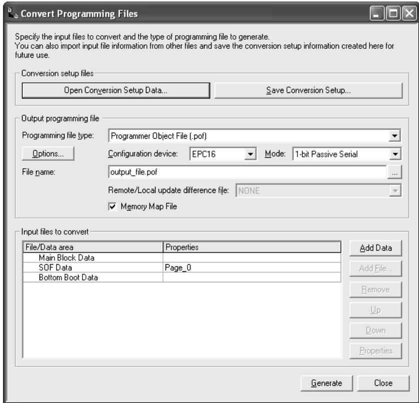
For a Programmer Object File for an EPC4, EPC8, or EPC16 configuration device, you can also specify the following information:
