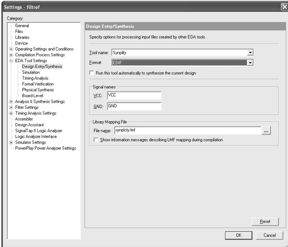
To run an EDA synthesis tool listed in the **Design Entry/Synthesis** page from within the Quartus II software, on the Processing menu, click **Start**, and then click **Start EDA Synthesis**. Many EDA tools also allow you to run the Quartus II software from within the EDA tool's GUI. Refer to your EDA tool documentation for more information.
