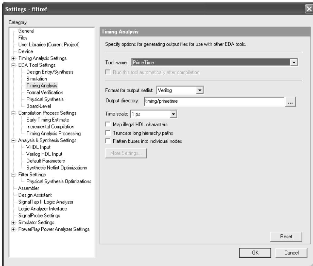
You can also generate the files by pointing to **Start** on the Processing menu, and then clicking **Start EDA Netlist Writer** after an initial compilation. If you are using the NativeLink feature, you can also run a timing analysis after an initial compilation by clicking **Run EDA Timing Analysis Tool** on the Tools menu.
