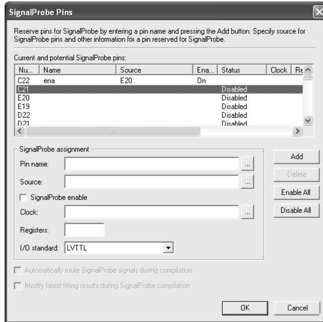
1. Perform a SignalProbe compilation, by pointing to Start on the Processing menu, and then clicking **Start SignalProbe Compilation**.
