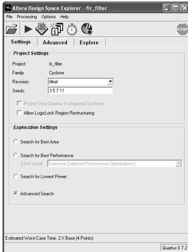
DSE provides several exploration modes, which are listed under **Exploration Settings** in the DSE window:
