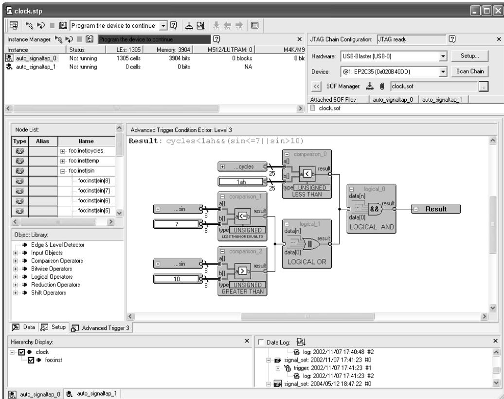
You can configure the logic analyzer with up to ten trigger levels, which help you view only the most significant data. You can specify four separate trigger positions: pre, center, post, and continuous. The trigger position allows you to specify the amount of data that should be acquired before the trigger and after.
