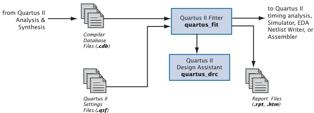
If you have made resource assignments in your design, the Fitter attempts to match those resource assignments with the resources on the device, tries to meet any other constraints you have set, and then attempts to optimize the remaining logic in the design. If you have not set any constraints on the design, the Fitter automatically optimizes it. If it cannot find a fit, the Fitter terminates compilation and issues an error message.
