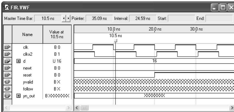
The Quartus II software supports waveform files in the Vector Waveform File (.vwf), Vector Table Output File (.tbl), Vector File (.vec), and Simulator Channel File (.scf) formats. You cannot edit a Simulator Channel File or Vector File in the Waveform Editor, but you can save it as a Vector Waveform File.
