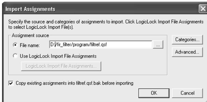
You can use this command to import a MAX+PLUS II Assignment & Configuration File, which contains MAX+PLUS II project assignments and settings, into your Quartus II project. You can also use this command to import settings and assignments from other projects created in the Quartus II software into your current project. For example, you can use this command to import pin assignments from a previous Quartus II project into the current Quartus II project.
