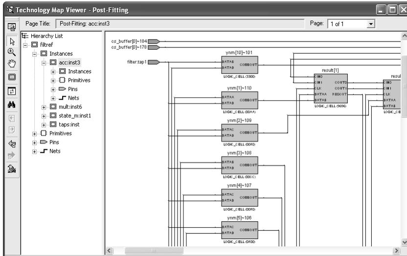
You can also use the Technology Map Viewer to display post-Analysis & Synthesis mapping and compare those results to the results from a full compilation. Display the results from Analysis & Synthesis by pointing to **Netlist Viewers** on the Tools menu, and then clicking **Technology Map Viewer (Post Mapping)**.
