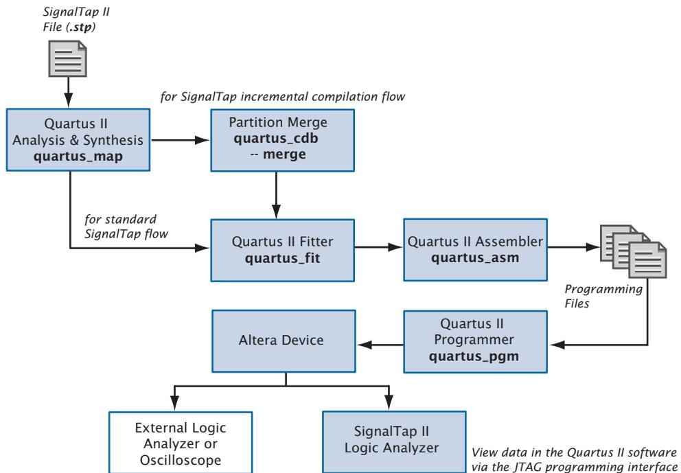
**Figure 2. SignalProbe Debugging Flow**
