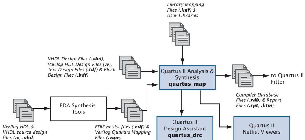
You can start a full compilation in the Quartus II software, which includes the Analysis & Synthesis module, or you can start Analysis & Synthesis separately. You can perform an Analysis & Elaboration to check a design for syntax and semantic errors without performing a complete Analysis & Synthesis or use the **Analyze Current File** command on the Processing menu to check a single design file for syntax errors.
