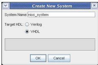
Figure 3: Naming a new system in SOPC Builder
