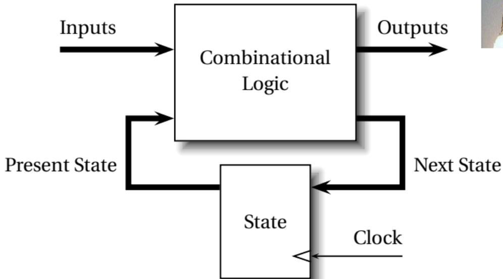
This is a *Mealy* FSM: outputs may depend directly on inputs.
