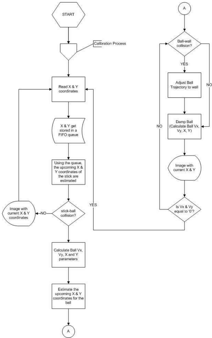
Figure 9: Primary Ball-Positioning Algorithm
