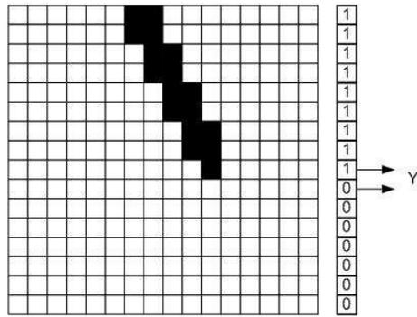
Figure 6: Vision System Algorithm Illustration - Cue cuts Top and Bottom Boundaries
