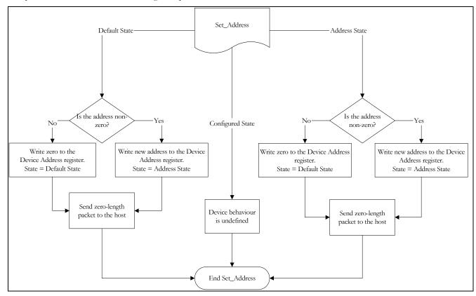
Figure 12-39: Flowchart of Set Address
