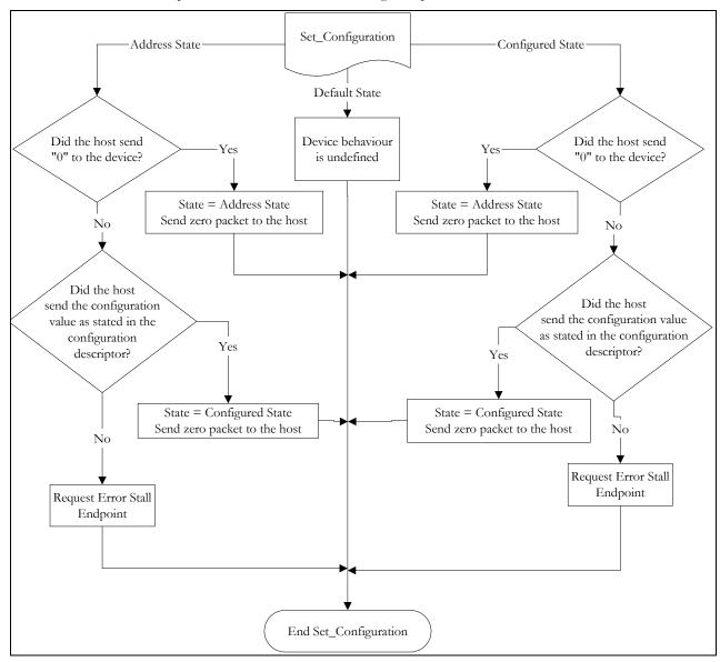
Figure 12-43: Flowchart of Set Configuration
