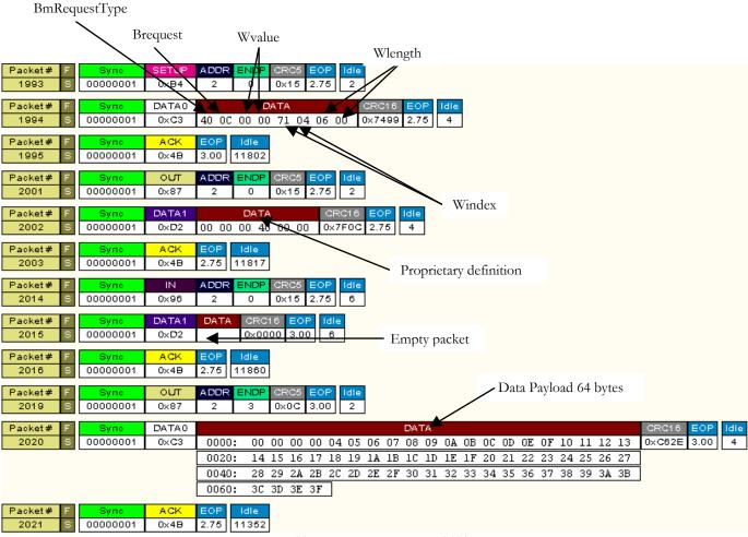
Figure 12-47: CATC Capture of a PIO OUT Transfer
