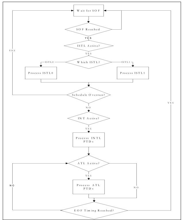
Figure 5-1: Flowchart of the Host Controller in the Operational State
