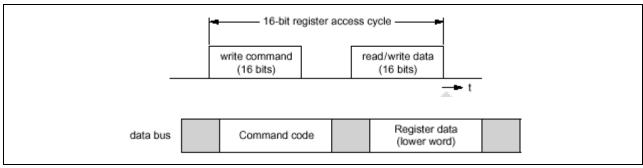
Figure 3-1: 16-Bit Register Access Cycle
