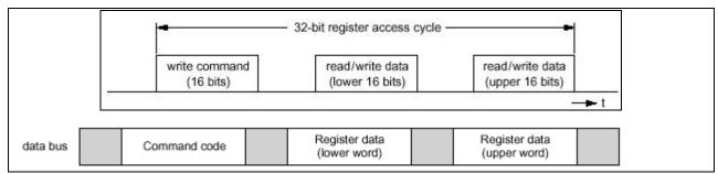
Figure 3-4: 32-Bit Register Access Cycle
