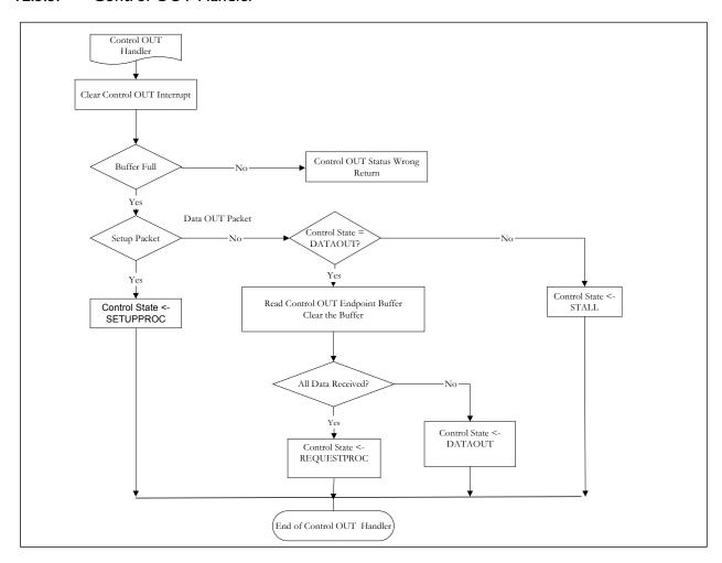
Figure 12-7: Flowchart of the Control OUT Handler
