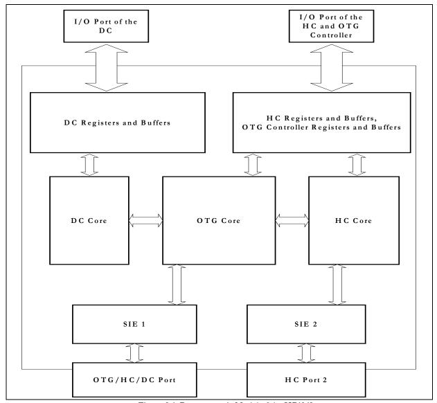
Figure 2-1: Programmer's Model of the ISP1362
