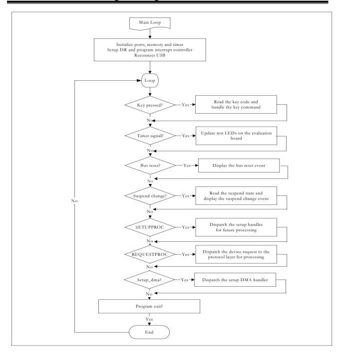
Figure 12-32: Flowchart of the Main Loop
