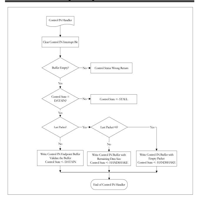
Figure 12-14: Flowchart of the Control IN Handler
