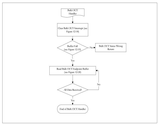
Figure 12-17: Flowchart of the Bulk OUT Handler
