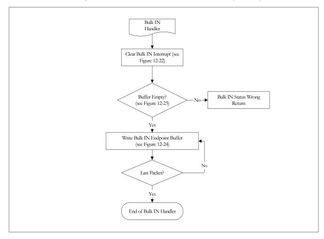
Figure 12-21: Flowchart of the Bulk IN Handler
