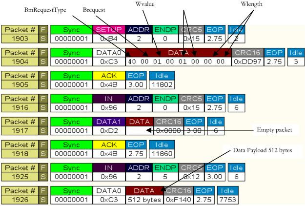
Figure 12-50: CATC Capture of an ISO IN Transfer
