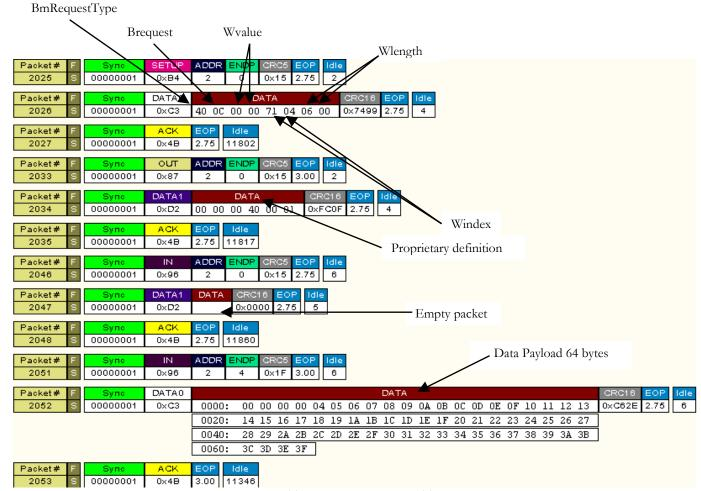
Figure 12-48: CATC Capture of a PIO IN Transfer
