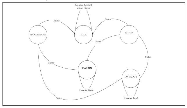
Figure 12-6: State Machine of the Control Transfer
