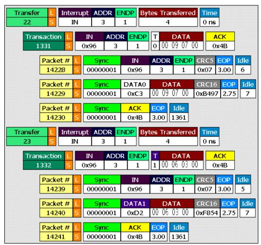
Figure 7-16: Snapshot of the Mouse Movement Data on the USB Bus
