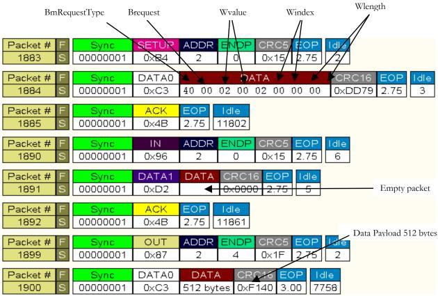
Figure 12-49: CATC Capture of an ISO OUT Transfer
