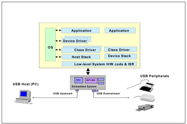
Figure 2-2: Software Model of the ISP1362
