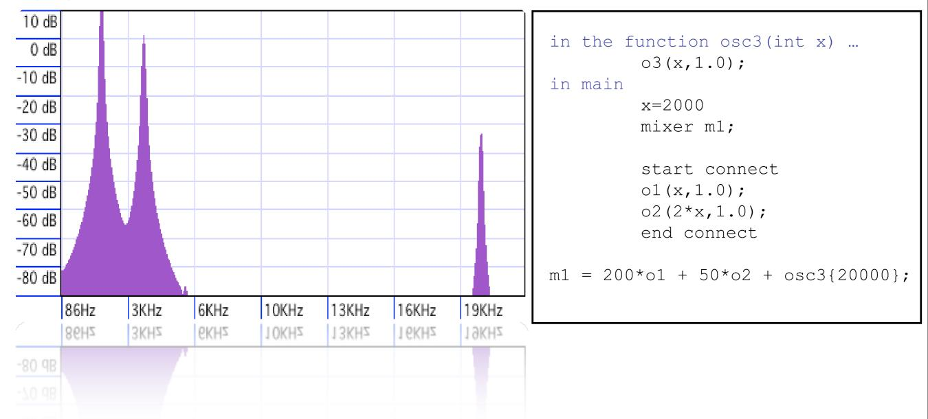
All oscillators, with increasing frequency (2kHz, 4kHz, 20kHz) and decreasing multiplicative factor are proportional in output amplitude length (200, 50, 1).
