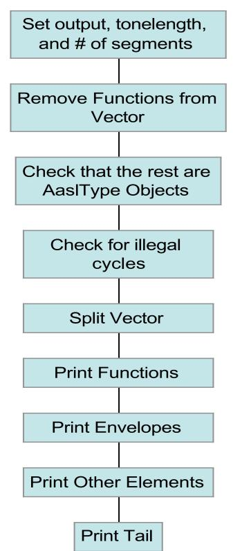
Illegal cycles: an oscillator indirectly end up attached to itself.
