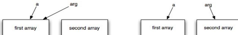
With the comment left in, the above code will evaluate to the left figure. If the line is uncommented, arg will point to a new Array, as shown in the right figure.
